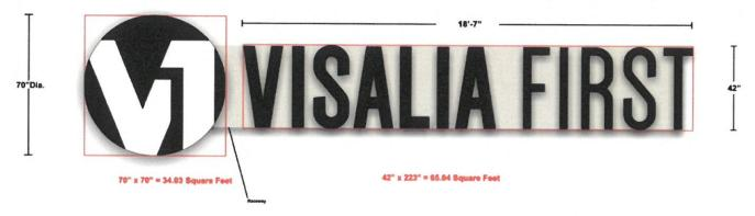
The proposed signs illustrated in Exhibit "B" represent two identical 100 square foot signs to be placed on separate wall frontages. The sign consists of letters (42" in height and 18'-7" in length totaling 65.04 square feet) and a circular logo (70" in height totaling 34.03 square feet).
