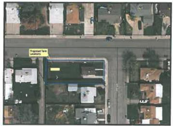
The improvements to the site will include new piping leading to the new GAC treatment tanks. Due to separation requirements and site constraints, the tanks will be located in the rear yard setback area. The tanks will be located ten feet from the rear property line and 15 feet from the side (north) property line, which coincides with the right-of-way with Sequoia Avenue.
