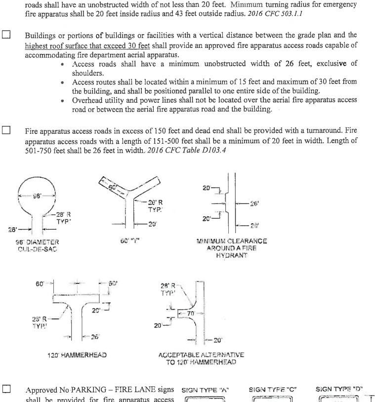
shall be provided for fire apparatus access roads to identify such roads or prohibit the obstruction thereof. Signs shall have a minimum dimension of 12 inches wide by 18 inches high and have red letters on a white reflective background. 2013 CFC 503.3/D103.6
