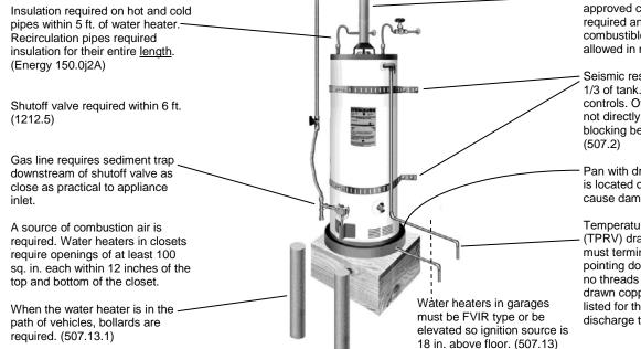
B Vent terminating min 1 ft. above roof in approved cap. Double-wall "B" vents are required and must have 1 in. clearance to combustibles. Single wall connectors are allowed in min. 6 in. clear to combustibles.
