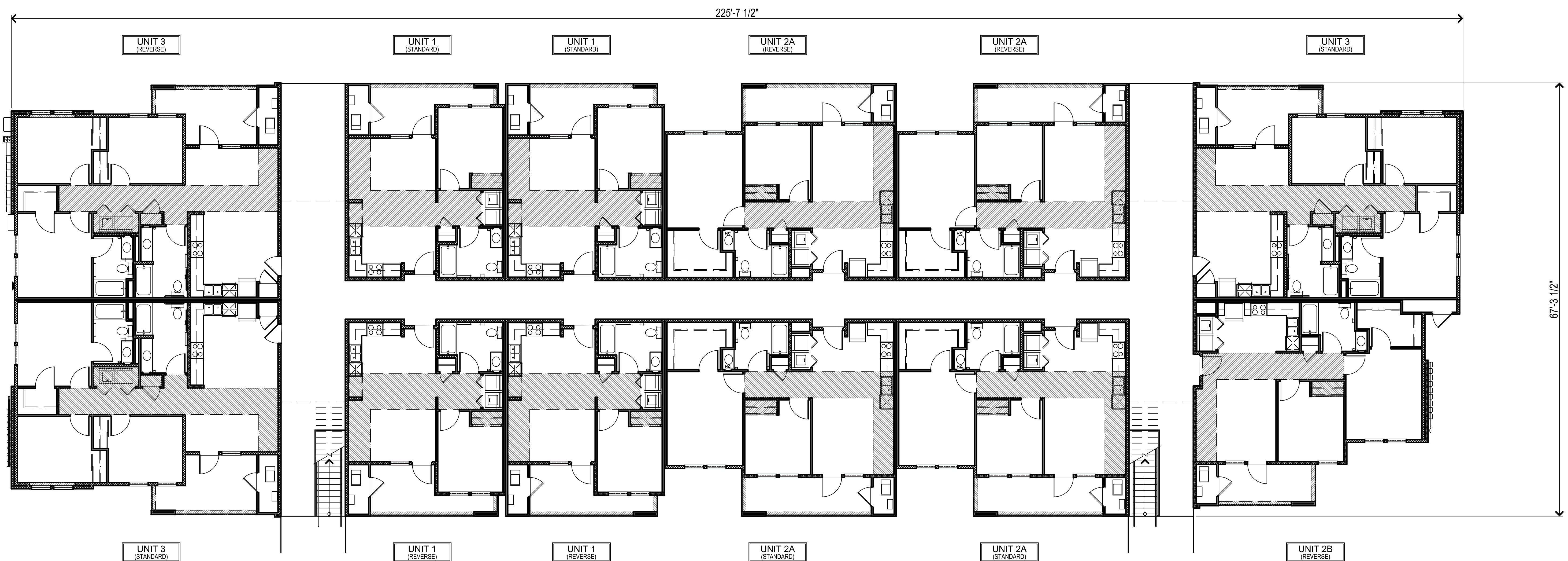
BUILDING TYPE 3s-36B (36 UNIT BLDG) - TYPICAL FLOOR PLAN
